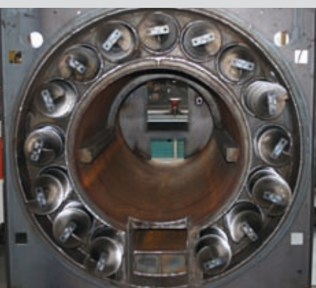
Generous heat exchanger with cleaning auger.
