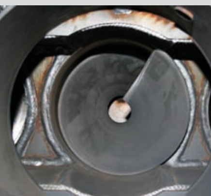
De-ashing augers for cleaning the heat exchanger.
