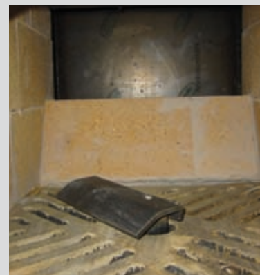
Stable cast grate with ash scraper.
