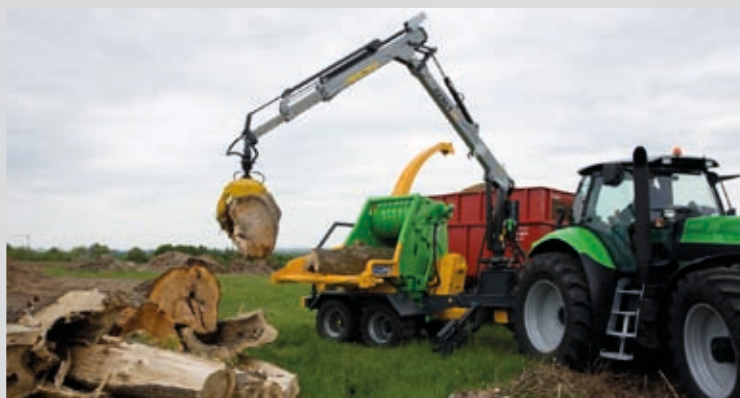
Heizohack crane-feed chipper for 50-80 cm diameter trunk.
